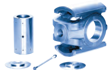
Ductile iron crossheads, babbitted shoe surface, full-floating crosshead pin with "through-bolt" and end caps
